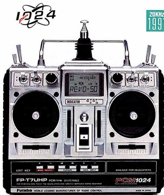
**7UHP/7 channel PCM 1024 Helicopter system.** R129DP receiver, five S5101 servos, computer LCD screen, ATV, dual rate, exponential, programmable mixing, timer, invert switch, hover memory, pitch mixing, tail rotor mixing, servo reverse, memory, trainer system, plug-in RF module 1000mAh receiver NiCd. 50 and 72MHz.
