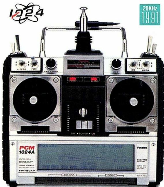
**9VA/9 Channel PCM 1024 Aircraft system.** R129DF receiver, four S5101 servos, LCD computer screen, ATV, AFR, ATR, programmable gang mixing, variable pitch propeller mixing, dual rate (3), exponential, adjustable VTR, timer, snap roll (3), servo reversing, mutual mixing, plug-in RF module, DSC. All NiCd. 50 and 72MHz. (Also available with four 9101 servos.)
