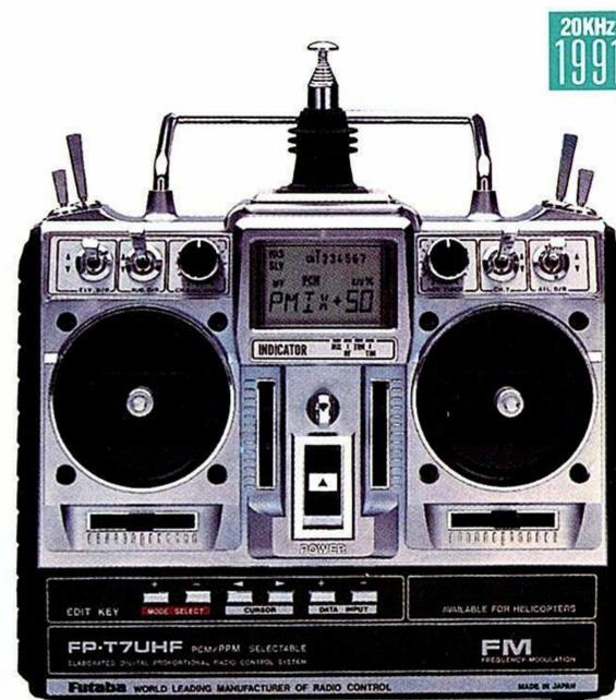
**7UHF/7 Channel FM Helicopter system.** R128DF receiver, four S5101 servos, computer LCD screen, ATV, dual rate, exponential, programmable mixing, timer, invert switch, hover memory, pitch mixing, tail rotor mixing, servo reverse, memory, trainer system, plug-in RF module 1000mAh receiver NiCd. 50 and 72MHz.
